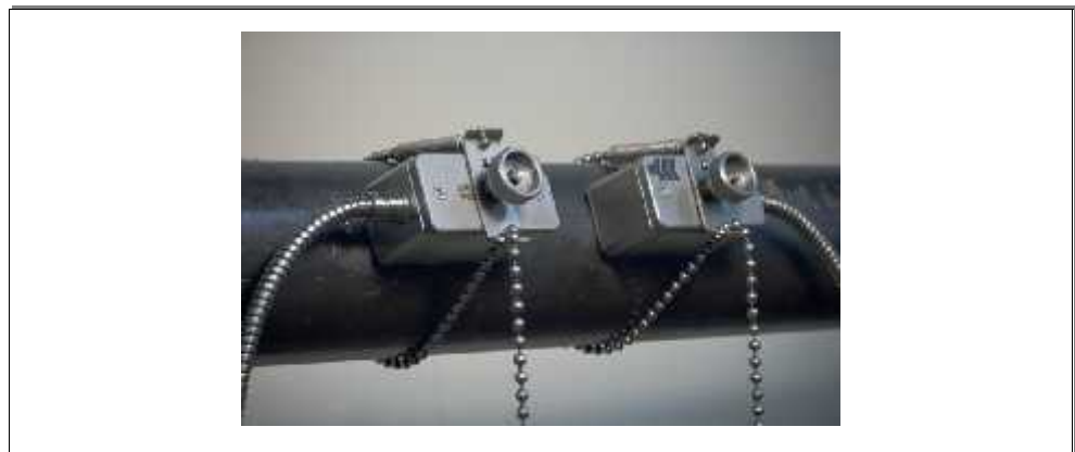
Illustration 7: Sensor mounting with clips and chains
