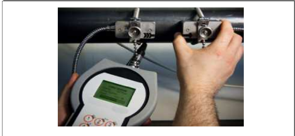
Illustration 6: Correct positioning of the sensors
